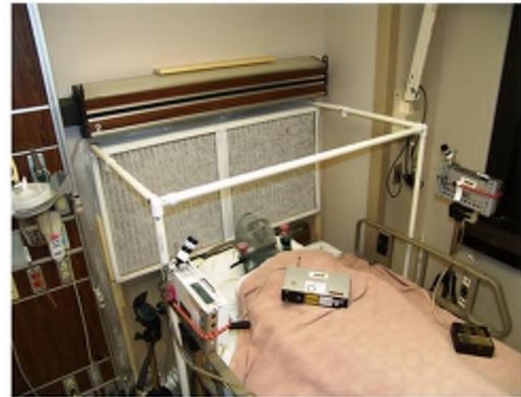
Figure 19. Photograph of ventilated headboard and hood frame as constructed for research at the Oklahoma City VA Medical Center.
